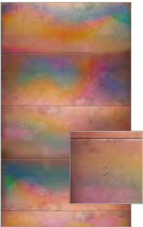
Heat Stressed Copper Plates
